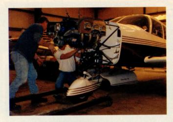
**Technicians install** Illtimate's overhauled engine. Note the newly painted firewall, and the blue crankcase and oil pan. The engine color will match an accent stripe on the final paint job. which will be provided by Dial **Eastern States** Aircraft Painting. Inc. of Cadiz, Ohio.
